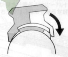
4 Fix firmly using an attached screw.
