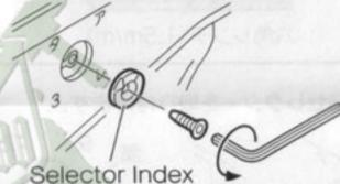
Use an attached screw and fix firmly.
